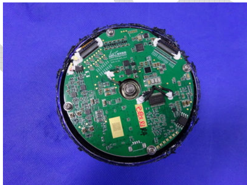
Fig.R14.7 After the test no water
