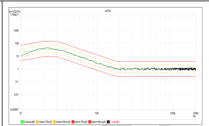
Fig.R07.14 Curves of vibration Z axis
