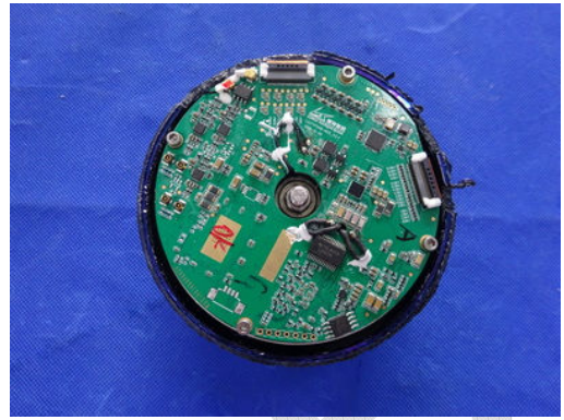
Fig.R12.10 After the test no salt solution inside
