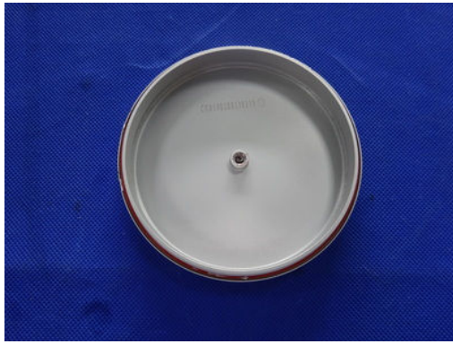
Fig.R12.9 After the test no salt solution inside
